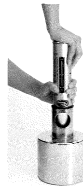
Fig. 3.1 Performance check of the concrete test hammer (model N/L shown)
