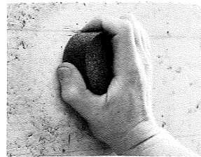
Fig. 2.1 Preparing the test surface
