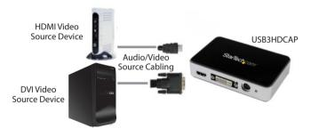
c. If your video source is VGA, use the included DVI to VGA video adapter to connect your VGA video source cabling to the DVI video input port on the USB3HDCAP (Please see the diagram on the next page for reference).
