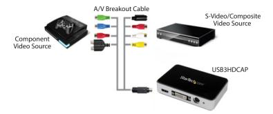
b. If your video source is HDMI or DVI, connect your audio/video source cabling directly to the HDMI audio/video input port or DVI video input port (respectively) on the USB3HDCAP.
